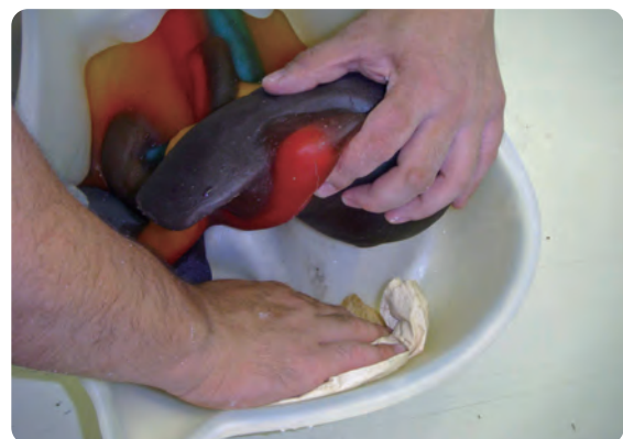
② Wipe the container walls and the phantom by soft cloth and make them dry before storage.
