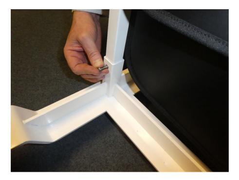
Insert screw and tighten bolt, and fit plastic cap.
