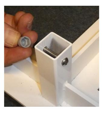
Remove plastic cap, nut and bolt from the Base with spanner and Allen key provided.
